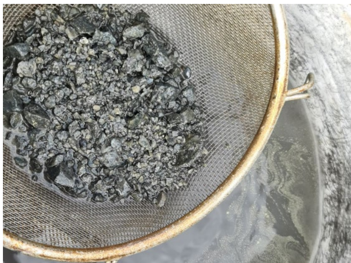
Figure 6: Copper-rich interval in RC drill chips showing abundant chalcopyrite in siliceous metasediment
