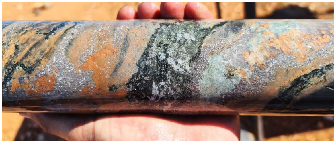
Figure 6: MI22RD05, ~179.7m – high grade cobaltite-rich zone (silver speckles) in strongly altered and deformed calcareous metasediment (HQ core)
