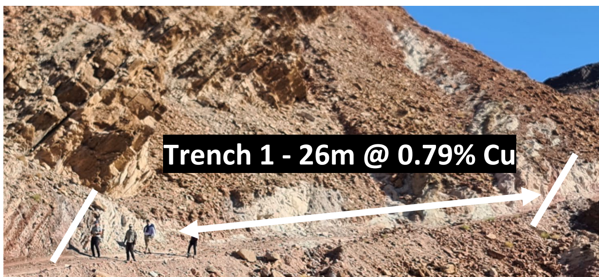
Figure 5: Malaqa North cutting showing 26m @ 0.79% Cu channel sampling interval. Note bounding red clay/shale units at either end
