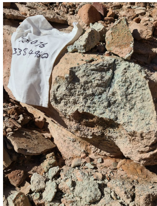
Figure 4: CuO (malachite) disseminated in soft clay-rich sandstone, Um el Amad area. 4.35% Cu.
