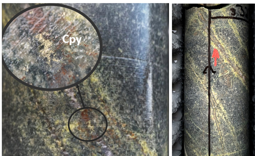
Photo 1. JUDD043 downhole depth of 175m - early quartz + molybdenite + chalcopyrite veins overprinted by strong pyrite + chlorite + epidote veins within a pervasive zone of propylitic alteration of gabbro host (NQ core).
