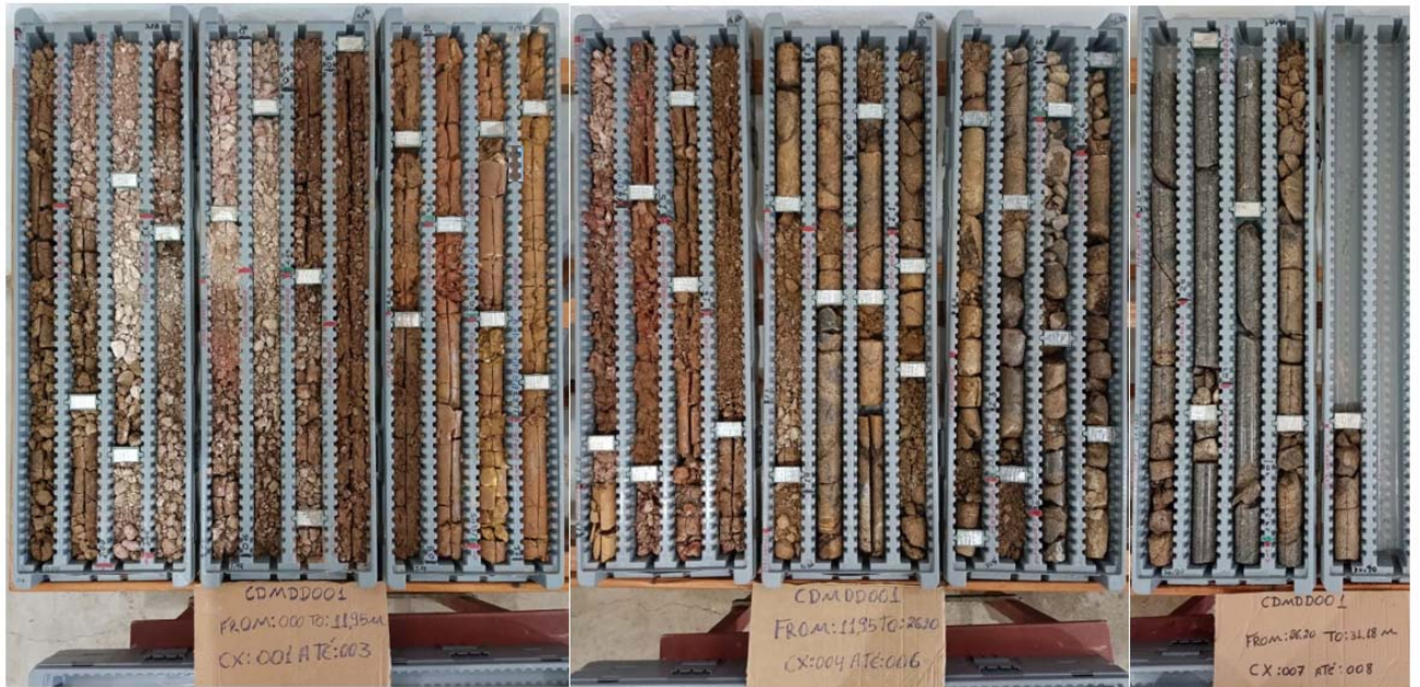
Figure 3. Core from the first diamond hole drilled at Capo Do Mel. This hole has a narrow soil horizon 0-1.4m and then a thick zone of Saprolitic clays until 26.6m. The hole finished in phonolite/syenite at 31.8m
