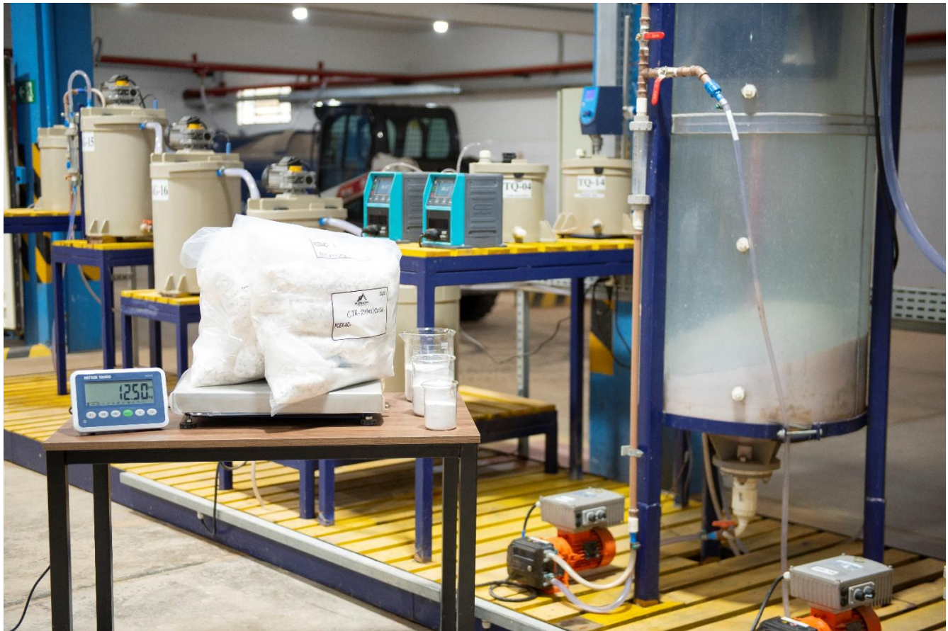
Figure 2 - Left Foreground - MREC produced over 4.5 days at 11.7 kg (dry) Right Foreground – White MREC bed (~20cm high) shown in thickener.
