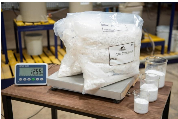
Figure 1: 11.7kg (12.55kg with packaging) of dry MREC produced over 4.5 days, i.e. 2.6kg/ day vs nameplate design of 1.8kg per day
