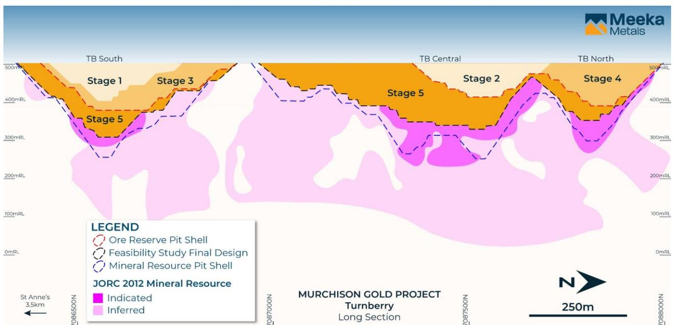
Figure 9 – Long Section showing open pit staging at Turnberry.
