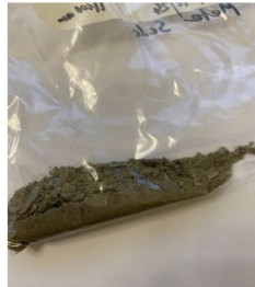
Scale recovered during meter cleaning 21 st Dec 2024 Awaiting results of analysis
