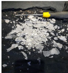
Scale recovered by drift & broach September 16 th 2024 Analysis indicates 100% barium sulfate
