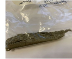
Scale recovered during meter cleaning 21 st Dec 2024 Awaiting results of analysis
