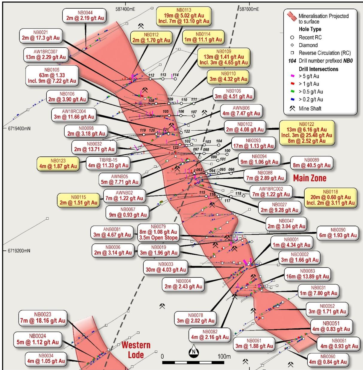
Figure 3: New Bendigo Drill Hole Collar Plan showing recent RC drill holes results (completed in 2022) in relation to previous drilling. Drill traces are projected to surface. Note the fault is inferred and further drilling is required to delineate mineralisation proximal to the fault New Bendigo. Recent highlighted intersections are shown as yellow callouts.
