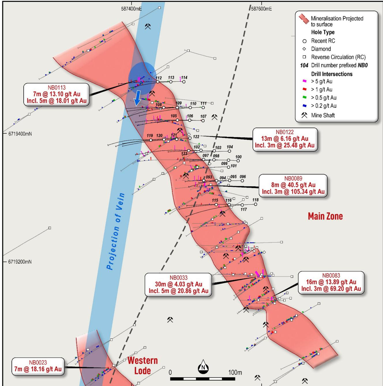
Figure 4: Projected strike of Au bearing Vein in DD Core from the NBD0005 containing visible gold at approximately 97m depth and high-grade Au intercepts within the road regional shear system (lower-grade envelope).
