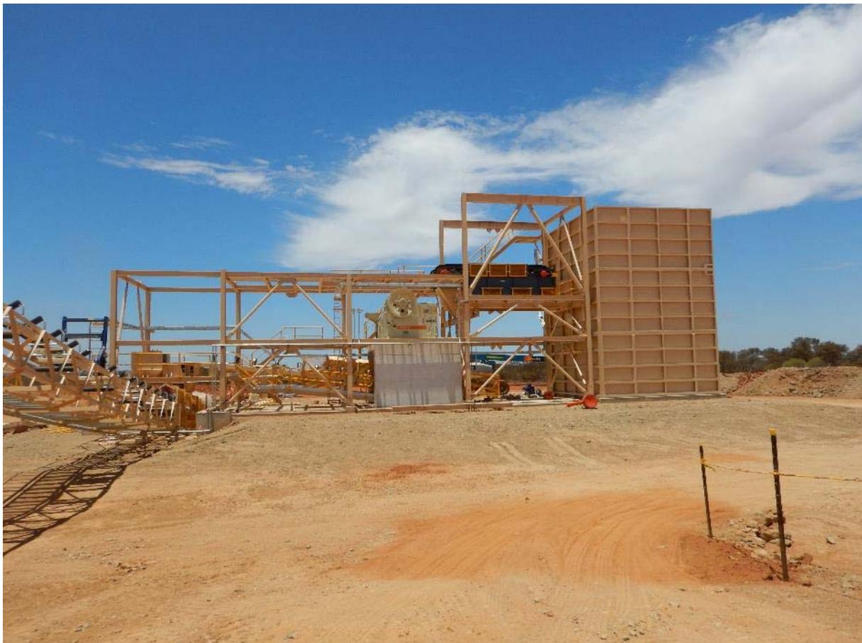
**Figure 1.** Primary crusher, ROM bin and apron feeder installed.
