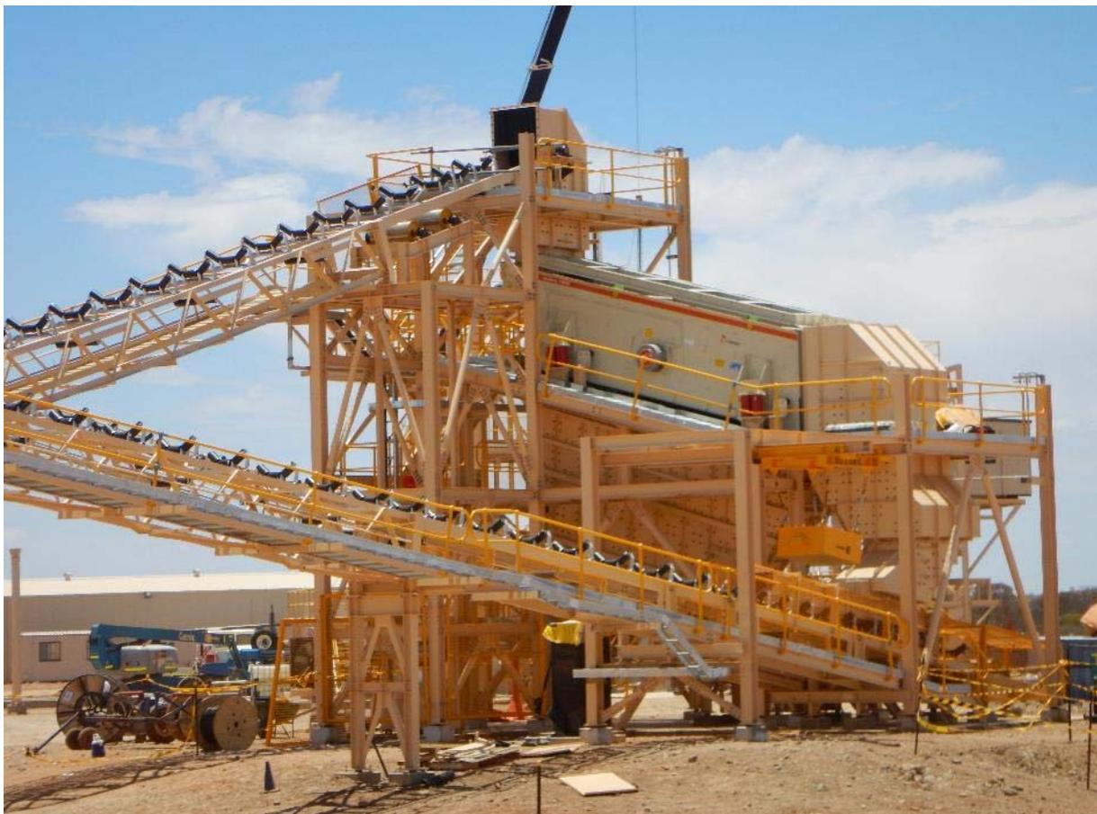
**Figure 3.** Crushing circuit screen installed.
