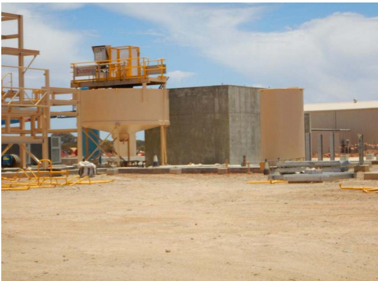
**Figure 7.** Concentrate thickener and concentrate bin.
