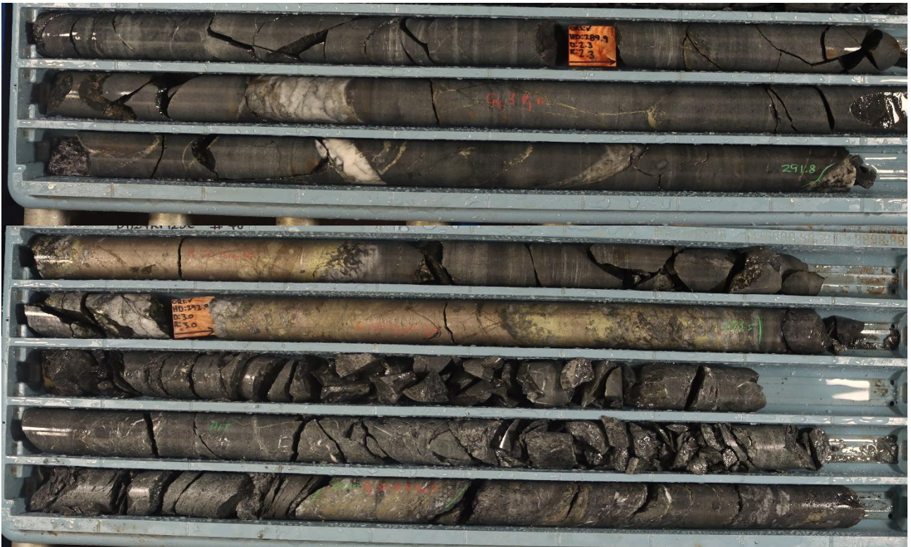
Figure 5: DD24KP1232 - ~1.7m interval containing two quartz sulphide veins from 291.8m comprising massive pyrrhotite (60%) and semi massive chalcocopyrite (20%) and pyrite (5%) within an intermediate volcanic host rock.
