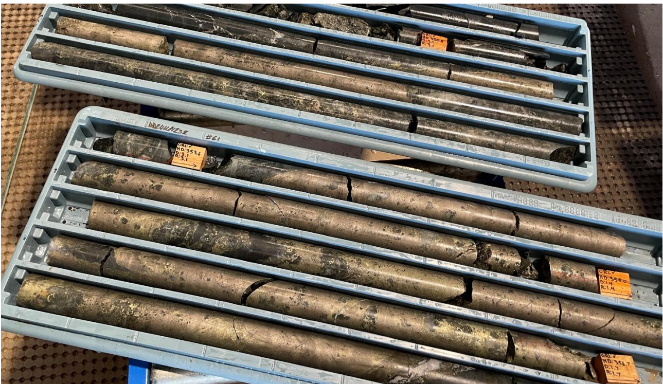
Figure 1: DD24KP1232 displaying semi massive to massive pyrrhotite-chalcopyrite mineralisation from approximately 353m downhole (assays pending).
