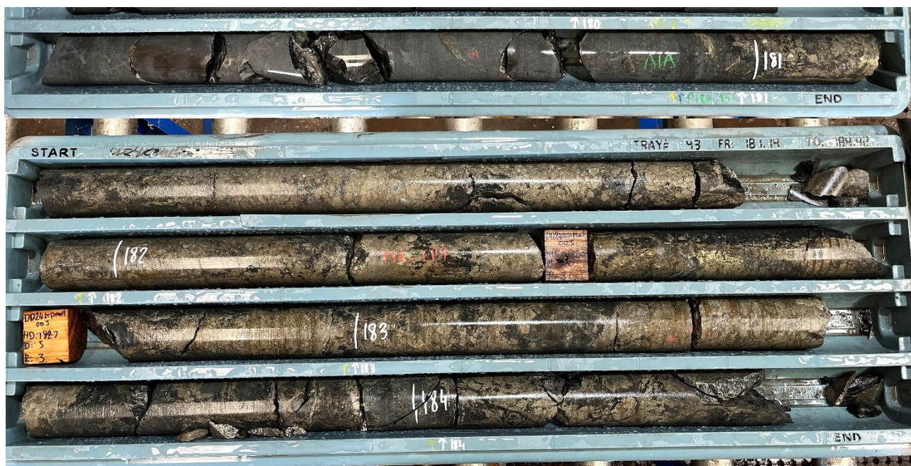
Figure 4: DD24KPMET003 displaying semi massive to massive pyrite-chalcopyrite mineralisation from approximately 181m downhole (assays pending).
