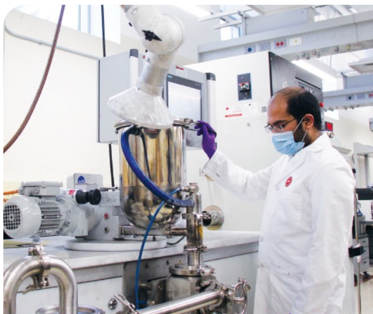
Particle engineering equipment held at C4V Labs in New York to upgrade Natural Graphite into Battery Anode Material
