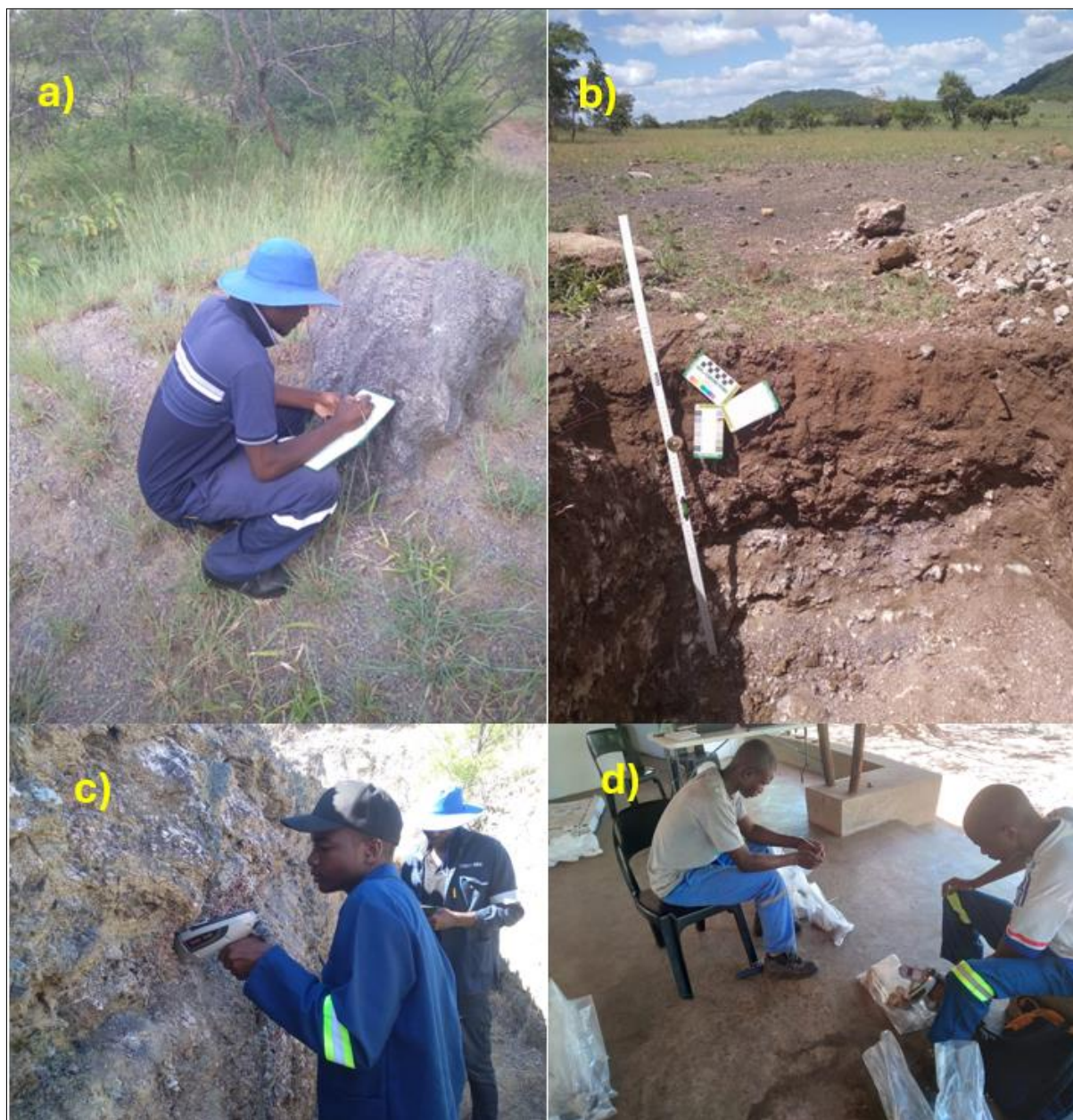
Figure 33: Images of exploration activities at Shawa. a) mapping taking place; b) pitting program to sample sub-crop during mapping; c) hand-held XRF analyses during field sampling and mapping; and d) hand-held XRF analyses at the sample handling facility of all rock and soil samples, with the rock samples to be analysed again by hand-held XRF after sample preparation (pulp samples).
