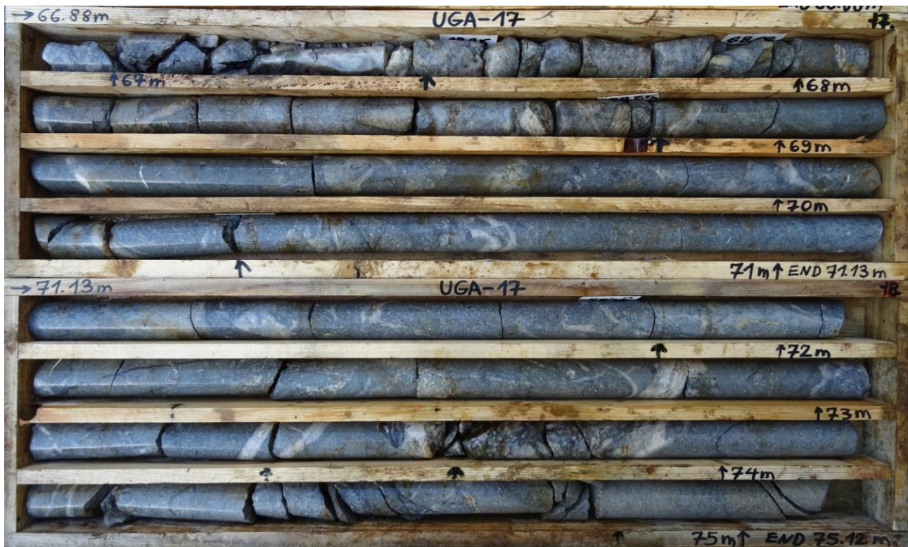
Figure 4: UGA-17 drill core; part of the interval from 51m to 97m (down-hole) showing quartz filled vein/stockwork/breccia structures, variably rich in fine to very fine grained sulphides (mainly pyrite/marcasite) and hosted within strongly argillic altered andesite host rock. Traces of visible gold identified at 73.75m in a ~25cm qtz vein
