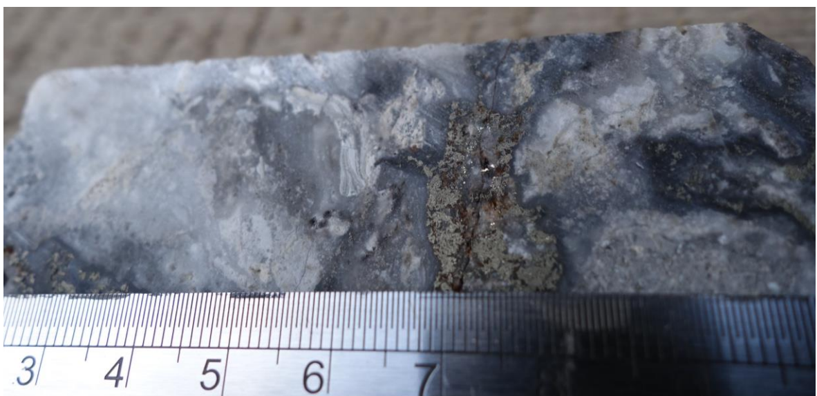
Figure 1: Visible gold in a ~25cm wide, drusy, fine grained, white to grey chalcidonic quartz-pyrite filled vein/stockwork zone at 73.75m in UGA-17. Visible gold found within a nest of pyrite upto 1.5cm wide and 2.5cm long
