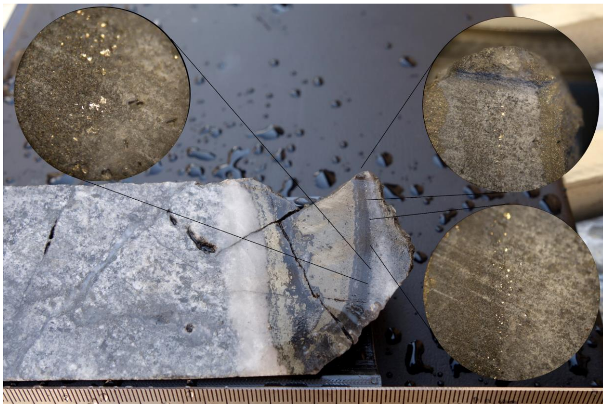
Figure 6: On this cut surface the Visible Gold is preserved as upto ~0.2mm sized grains within a ~5cm wide, grey-white, drusy quartz veinlet filled by fine-grained disseminated to semi-massive pyrite/marcasite crystals at 130.4m in UGA-41. Field of view of the right two magnified inset images is ~10mm across (x20) and the field of view of left magnified inset image is ~4mm across (x40).
