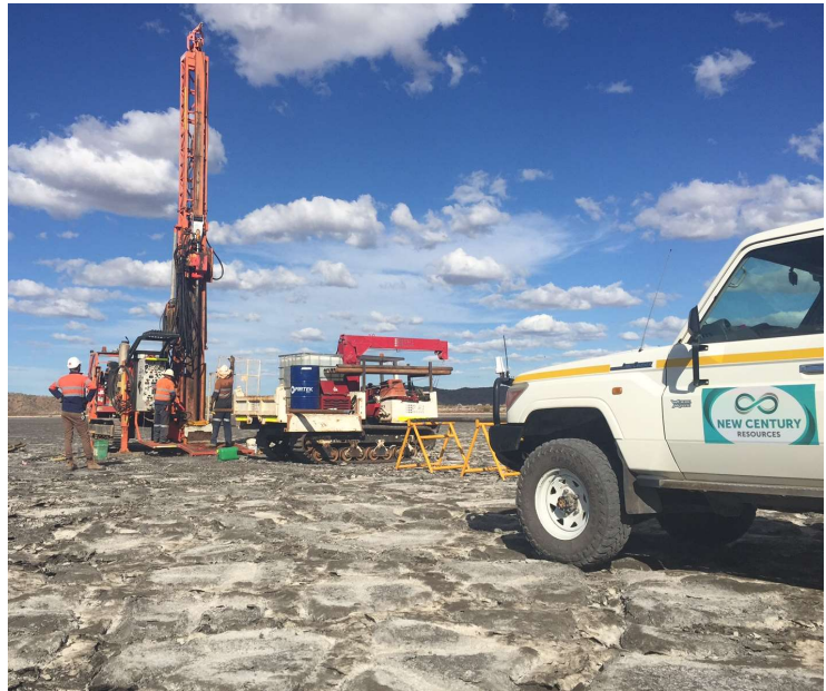
Figure 6: Tailings drilling at the Century Zinc Mine
