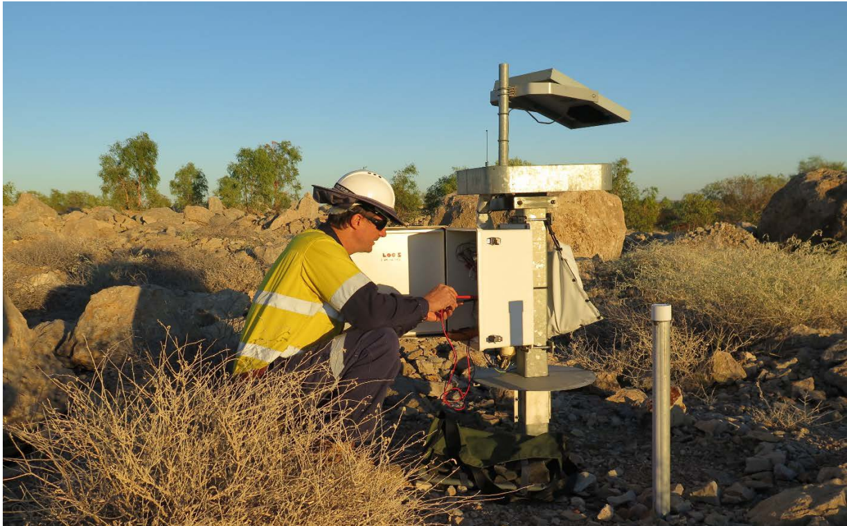
Figure 1: Waste rock dump cover monitoring systems, collecting performance data on waste rock rehabilitation at the Century Zinc Mine
