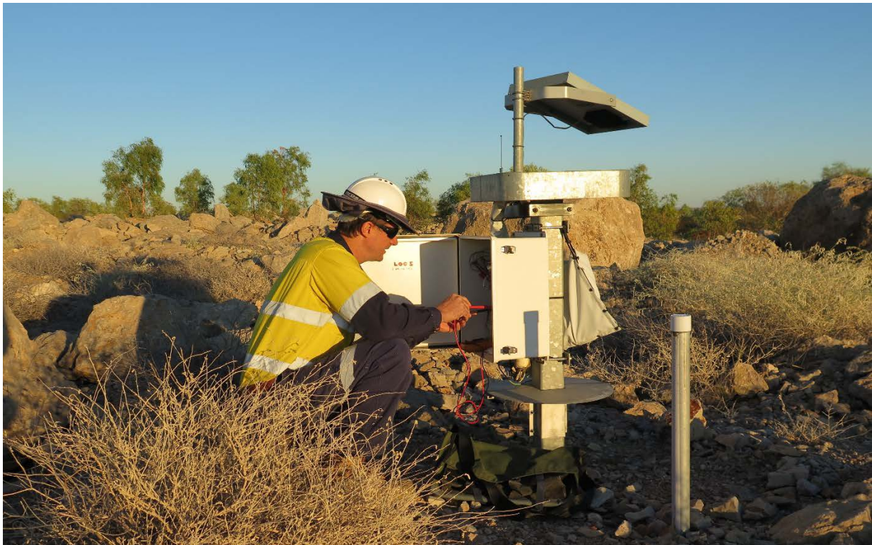
Figure 3: Waste rock dump cover monitoring systems, collecting performance data on waste rock rehabilitation at the Century Zinc Mine
