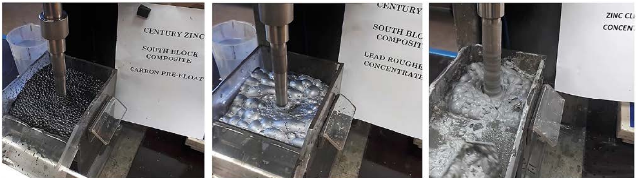
Figure 12: Progressive flotation of the South Block ore samples, with upfront carbon pre-float (left) followed by lead concentrate flotation (middle) and final zinc concentrate flotation (right)
