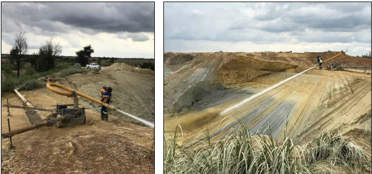
Figure 5: Ergo Mine hydraulic mining operations at one of the numerous tailings extraction locations (25Mtpa)
