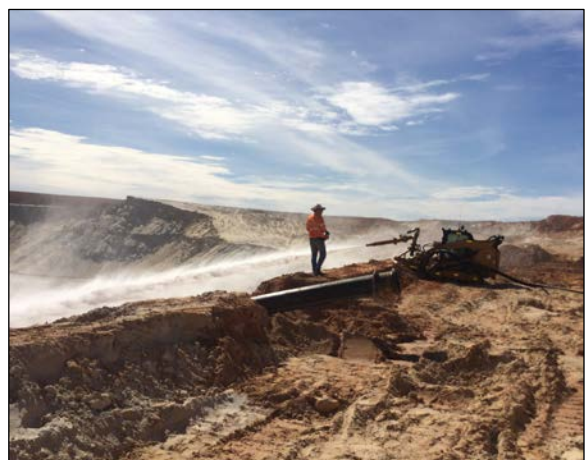
Figure 3: NPE remote controlled track mounted hydraulic mining cannons to be used at Century
