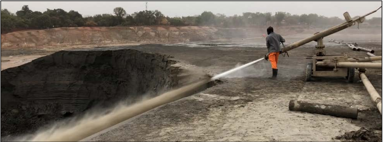
Figure 6: Morlia Gold Mine hydraulic mining operations (15Mtpa)
