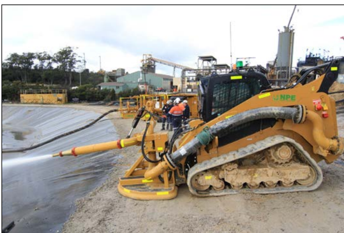
Figure 3: NPE remote controlled track mounted hydraulic mining cannons to be used at Century
