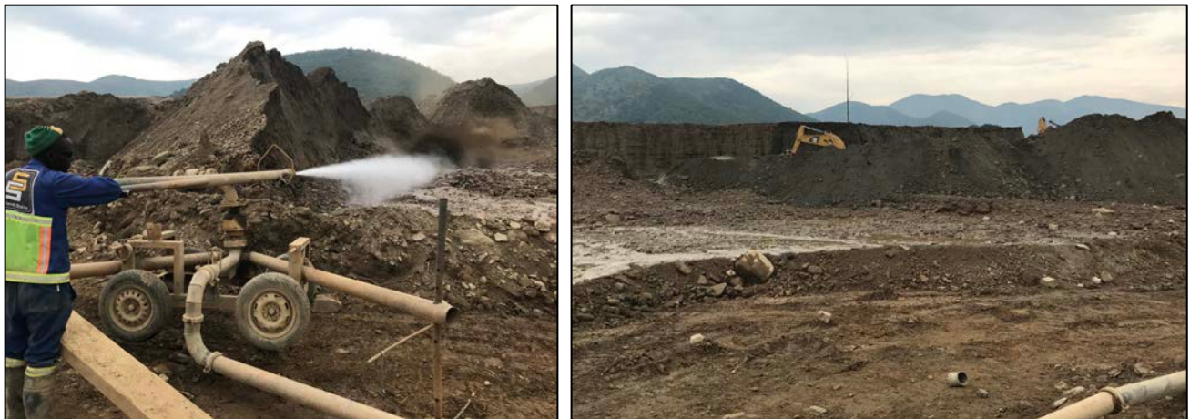
Figure 10: BTRP hydraulic mining of mechanically stacked dry tailings and waste dumps (1.2Mtpa)
