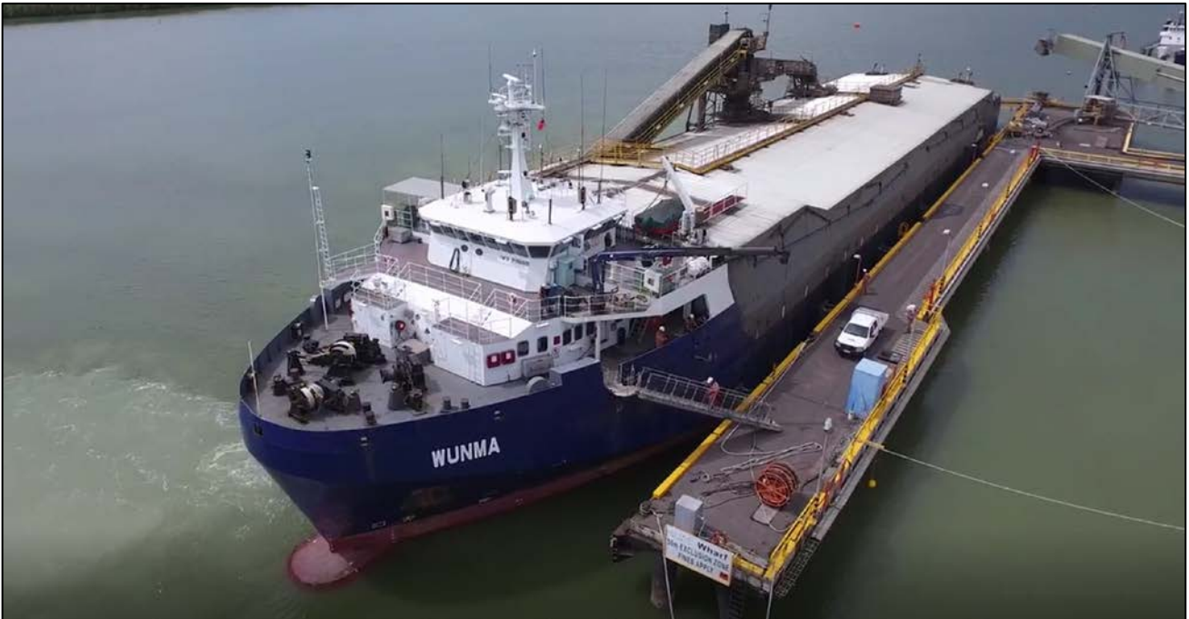
Figure 3: The M.V. Wunma, New Century's 114m long, 5,000t capacity transshipment vessel. The M.V. Wunma is presently docked at the Port of Papua New Guinea and is scheduled for return to Karumba in Q3 2018 in line with first shipments
