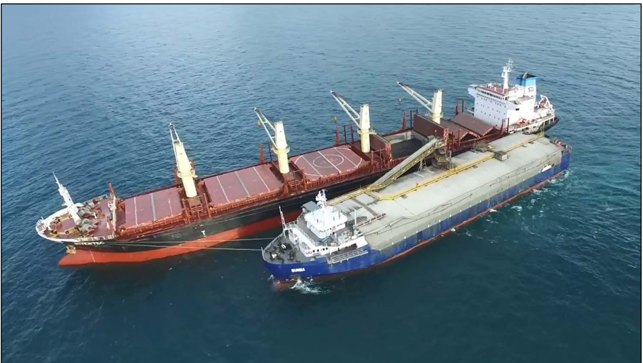
Figure 4: Historical operations of the W.V. Wunma, loading zinc concentrate into a bulk cargo export vessel ~20km offshore for transport to smelters around the world
