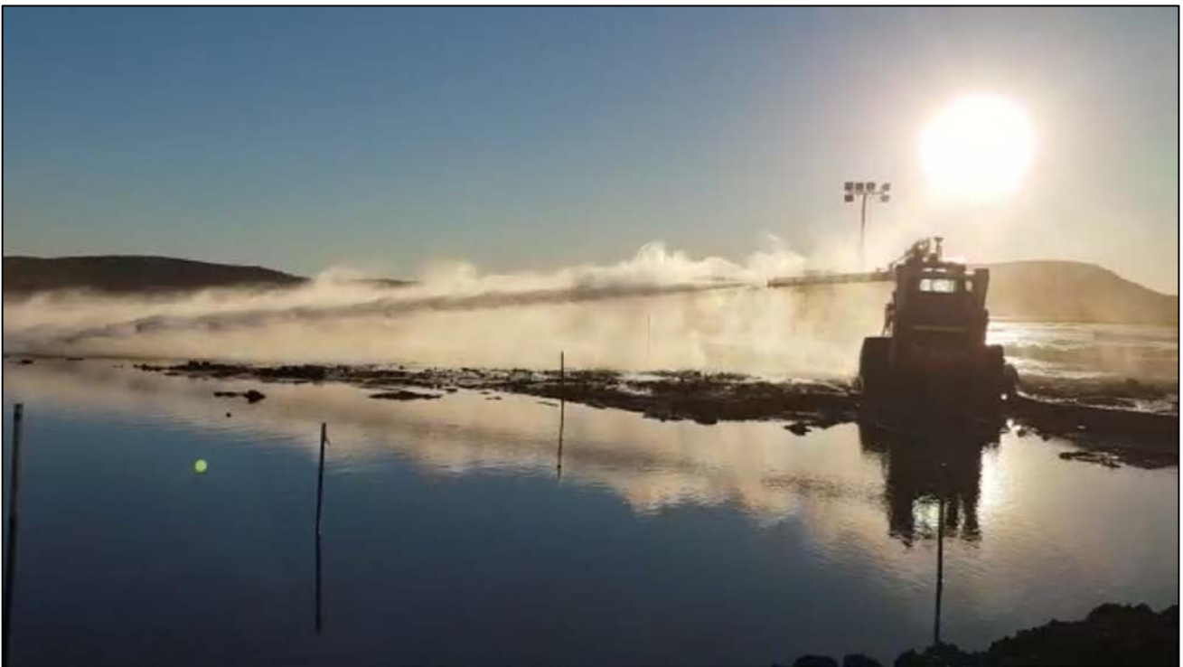
Figure 1: Hydraulic mining operations underway at the Century Zinc Mine
