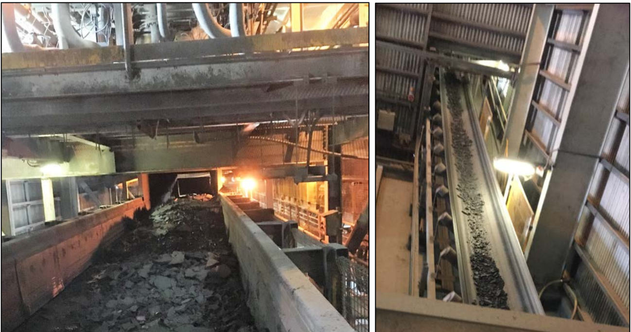
Figures 4 & 5: Pressed zinc concentrate discharged onto the conveyor belt below the filter press (left) and conveyor transport of the product to the concentrate storage shed (right) at the Karumba Port Facility
