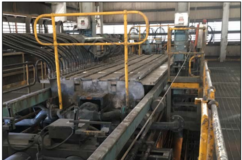
Figures 8 & 9: Zinc concentrate slurry entering the concentrate thickener from the slurry pipeline (left) and through one of the five filter presses (right) at the Karumba Port Facility
