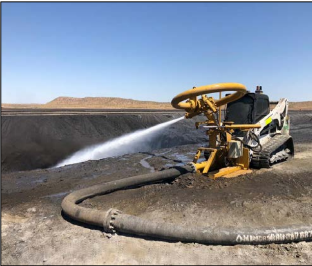
Figures 3 & 4: Hydraulic miner in operation (left) and the two hydraulic miners cutting the main trench on the Century Tailings Deposit (right)
