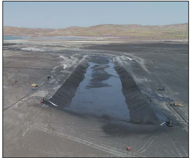
Figures 3 & 4: Hydraulic miner in operation (left) and the two hydraulic miners cutting the main trench on the Century Tailings Deposit (right)
