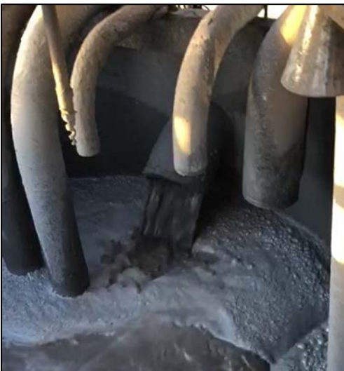
Figures 8 & 9: Zinc concentrate slurry entering the concentrate thickener from the slurry pipeline (left) and through one of the five filter presses (right) at the Karumba Port Facility
