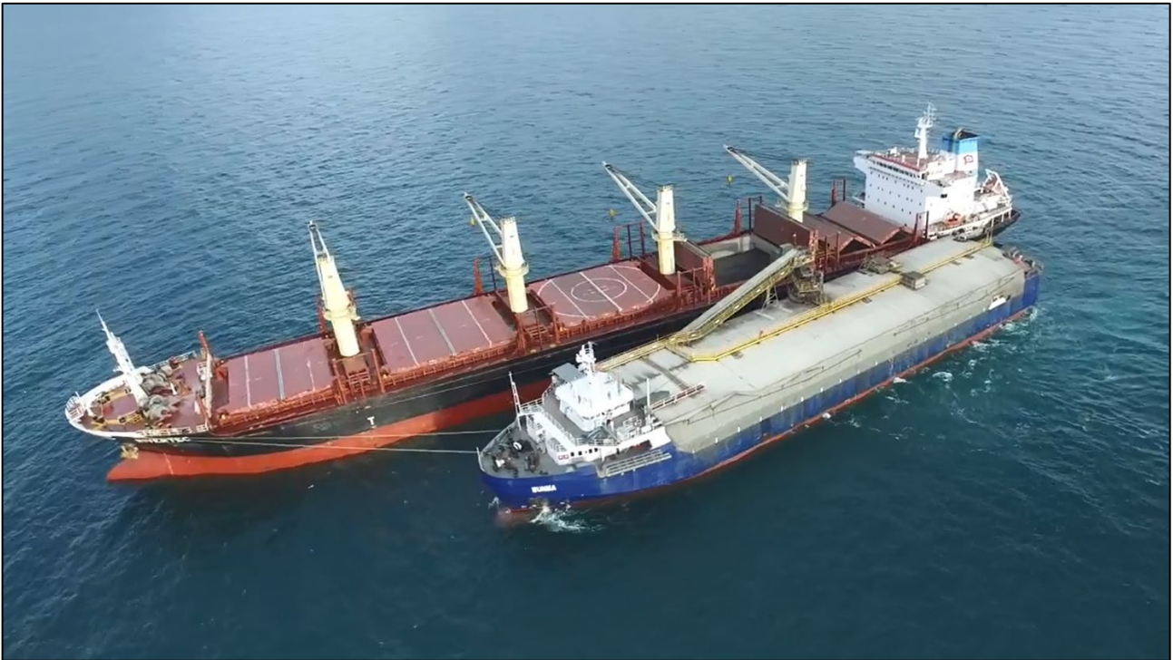
Figure 5: Example historical operations of the WV Wunma, loading zinc concentrate into a bulk cargo export vessel ~20km offshore for transport to smelters around the world
