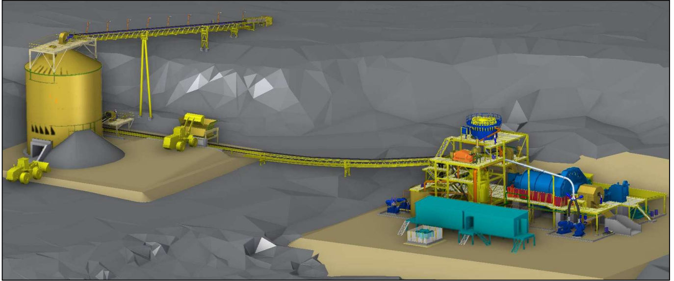
Figure 3: Fine ore bin & ball mill grinding circuit layout
