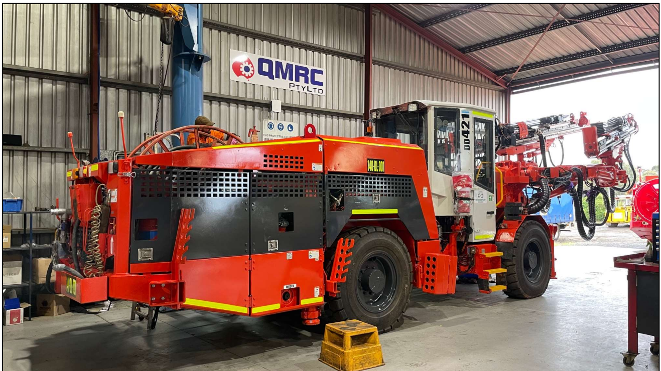
Figure 4: Sandvik DD421 Development Drill in the final stages of full rebuild
