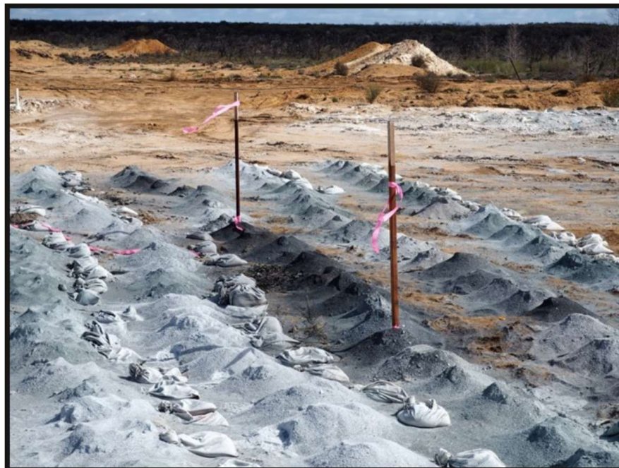
Figure 1 – NRRC124 R/C Drill piles, black material represents massive sulphide intersections (128-138m marked by wooden pegs).
