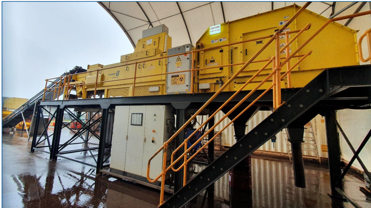
Figure 3: Steinert's KSS FLI XT Sensor Sorter used for sorting the NickelSearch ore.
