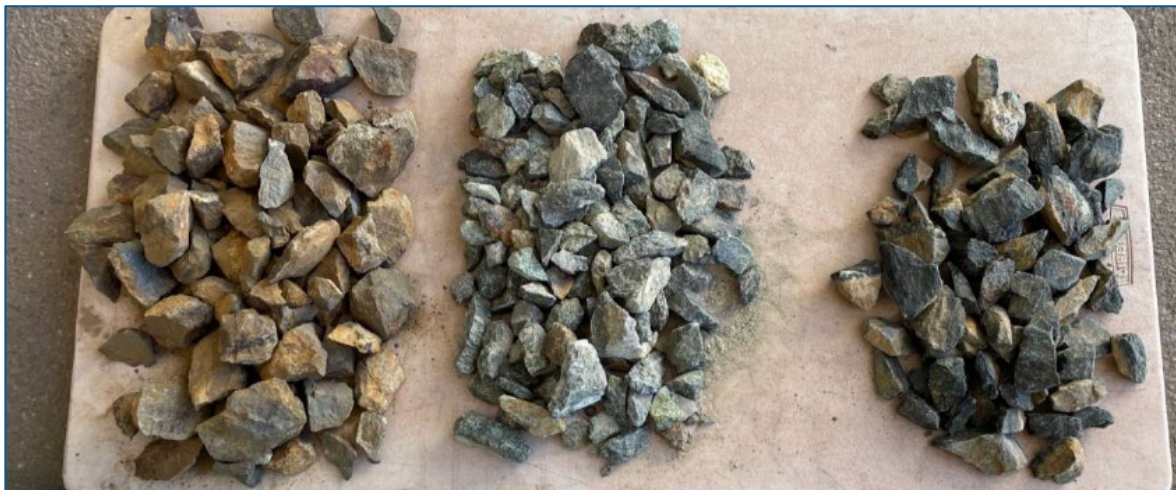
Figure 2: Hand selected samples of high-grade, low-grade, and waste rocks from site and used for identifying a 'signature' for sorting.
