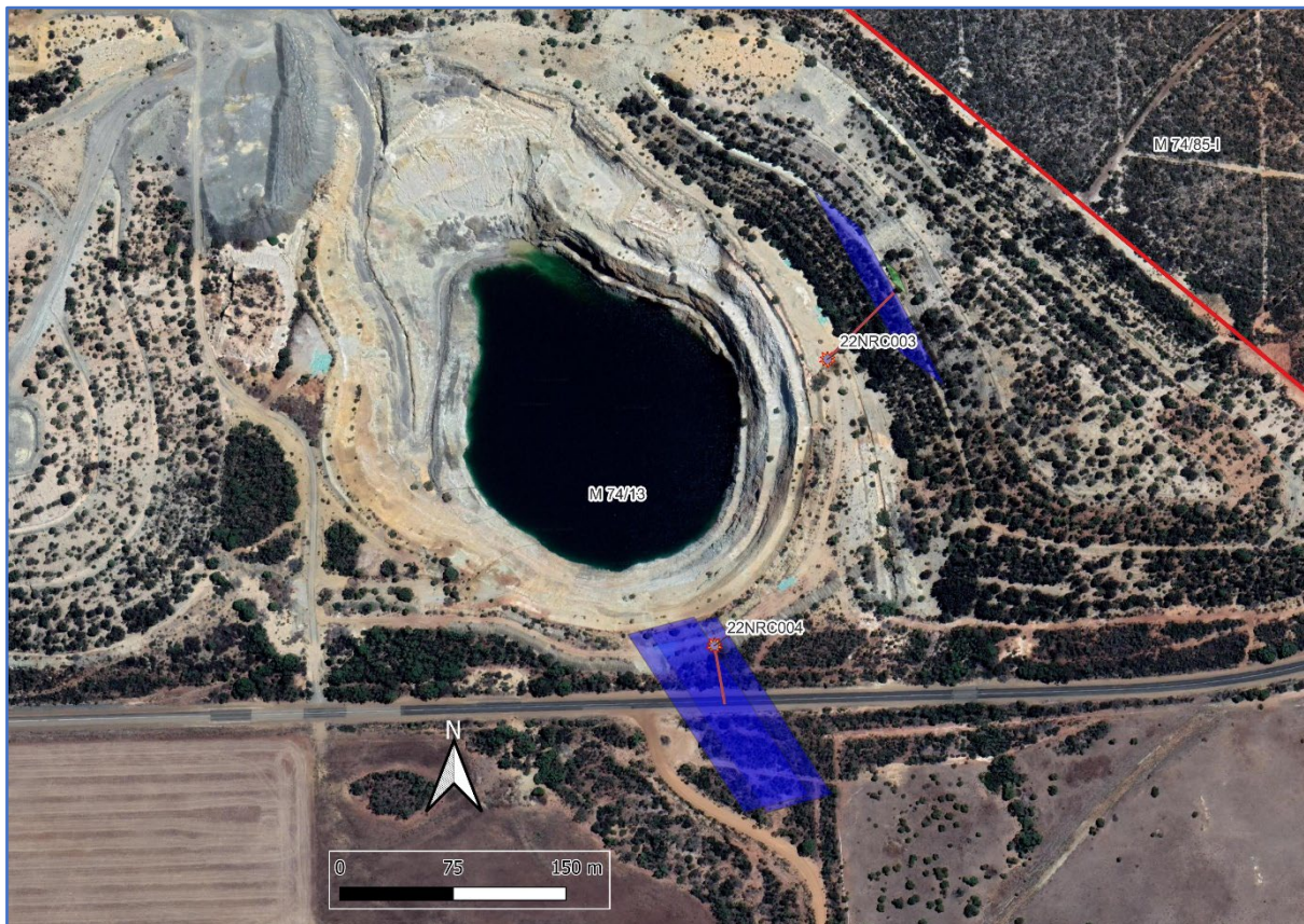
Figure 3: Recent drilling at RAV8 shown by red drill traces and blue DHEM plates.
