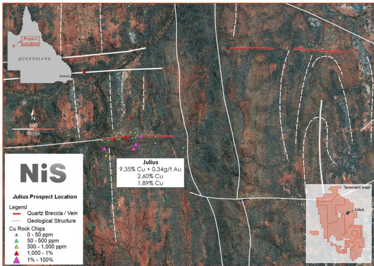
Figure 10: Julius Prospect Plan View (refer to Appendix G for chip samples details)
