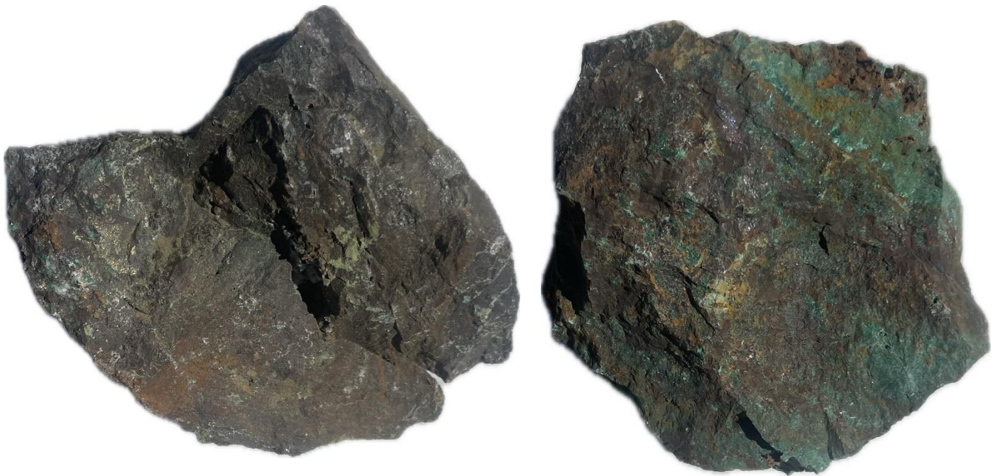
Figure 2: Rock Chips CSR001(11.3% Cu & 0.21g/t Au) (left) and CSR002 (24.8% Cu & 1.23g/t Au)(Right)
