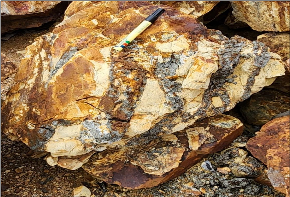
Figure 4: Sulphide Veining in Oversize
