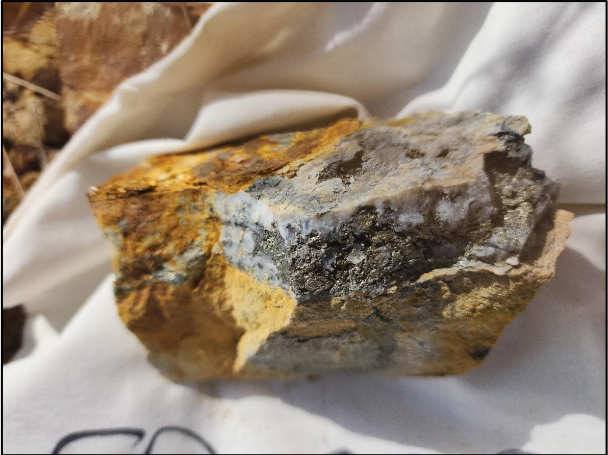
Figure 3: FF002 Showing pyrite sulphides in qtz vein (72.5g/t Au)
