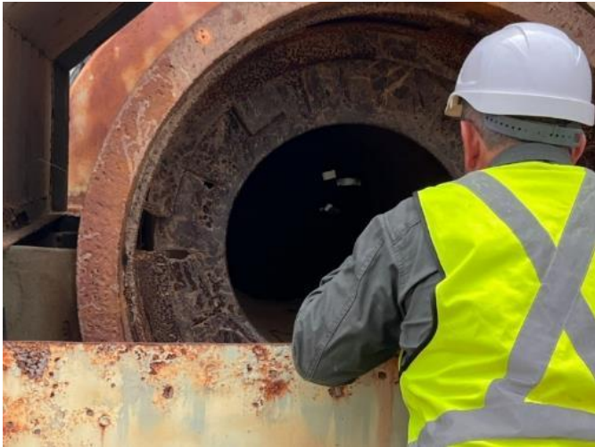
NMR Personnel supervising the confined space Mill Liner Measurement
