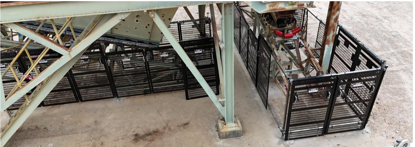
Guarding Panel Installed Across All Conveyors
