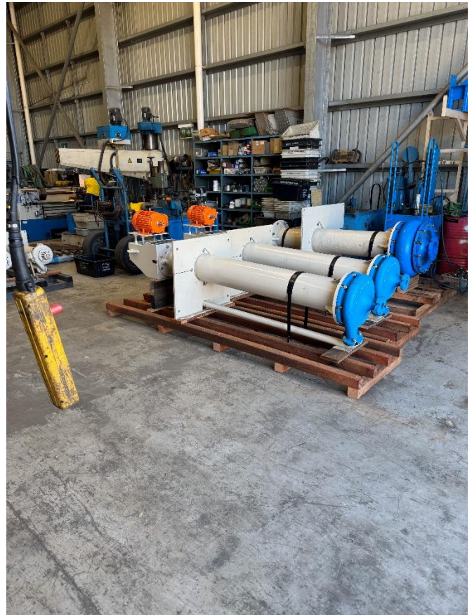
New Austral Carbon Transfer Pump & Components Completed and Ready for Dispatch
