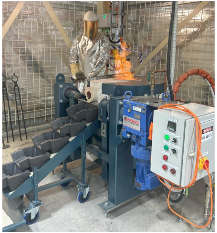
Figure 3: Operator in full protective gear oversees the controlled pour of molten gold during NMR's first trial at the Blackjack Gold Project
