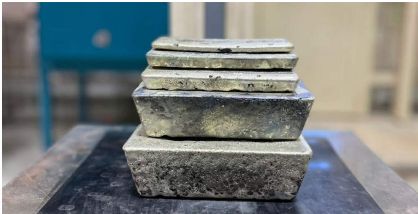
Figure 2: Gold doré bars produced from the latest Blackjack smelts on 14 September 2025.
