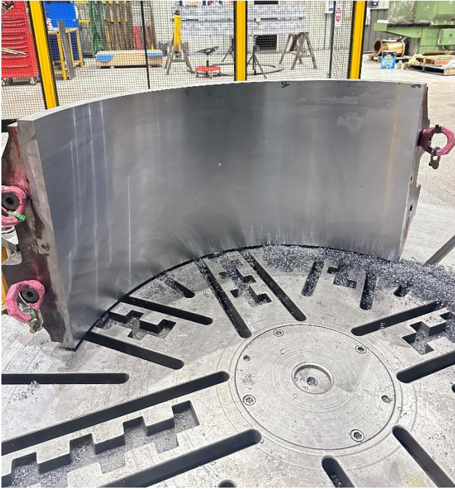
Figure 5a: Bearing white metal reline
