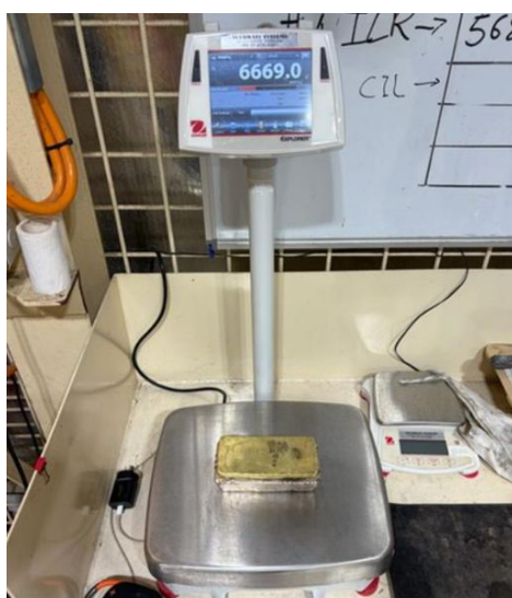
Figure 2: Total 214oz (6,669g) doré bars BJM049 and BJM050 – smelted at Blackjack on 8 th April 2026. Internal assay returned BJM049 at 78% purity.
