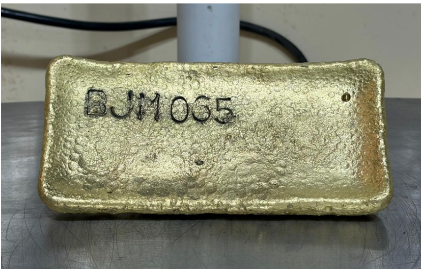
Figure 1: Gold doré bar BJM065 (88 oz doré), one of three doré bars (BJM065–067) produced during the 14 June 2026 smelt campaign, which yielded a combined total of 397.8 oz.
