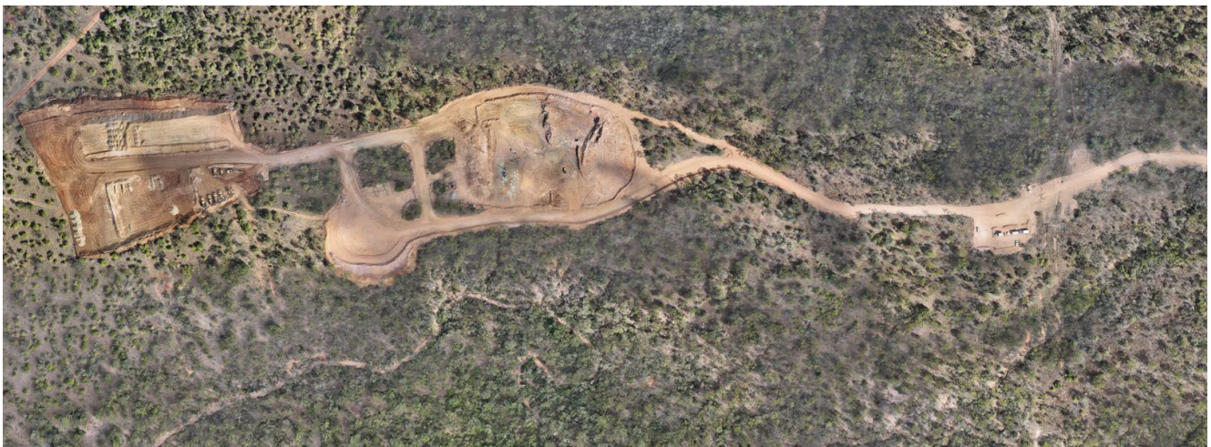
Figure 4: Mining activities at Podosky continue to advance on schedule, with waste removal progressing on Flitch 275 and the next production blast planned for Bench 267.5-01 on 25 June 2026.
