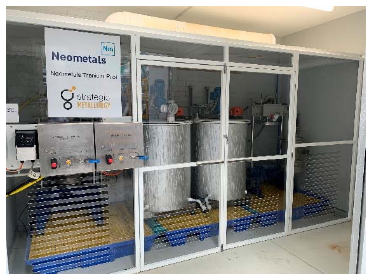
Figure 2 – Neometals Titanium leach and hydrolysate production reactors at Strategic Metallurgy, Perth
