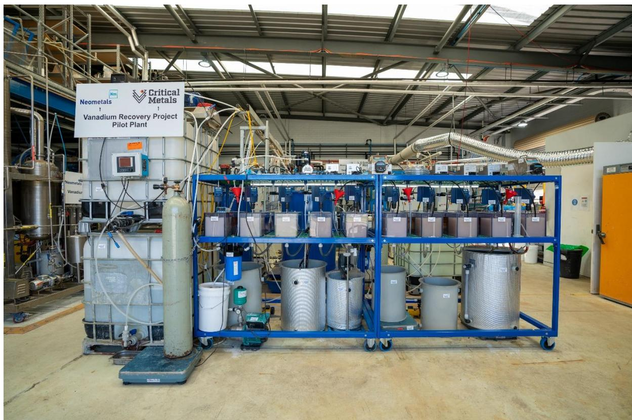
Figure 2 – Solvent Extraction section of Pilot Plant
