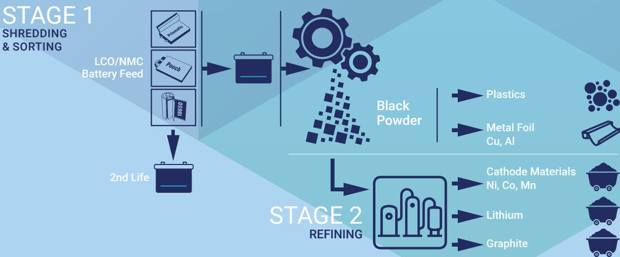
Figure 2 - High level flowsheet showing the materials generated from Feed Preparation and Hydrometallurgical Processing stages.
