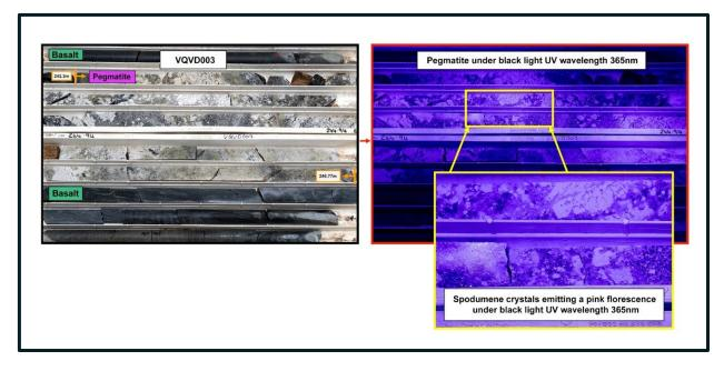
**Figure 1 –** Diamond Core from VQVD003 showing pegmatite intercepted between 242.3 – 246.77m under UV wavelength 365nm (blacklight). Spodumene fluoresces orange-pink under UV light from 242.3 – 245.5m.
