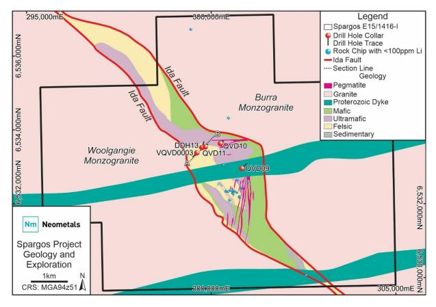
Figure 3 - Spargos Geology with Field Mapping and Lithium Exploration. Location of Section 1 shown on map.
