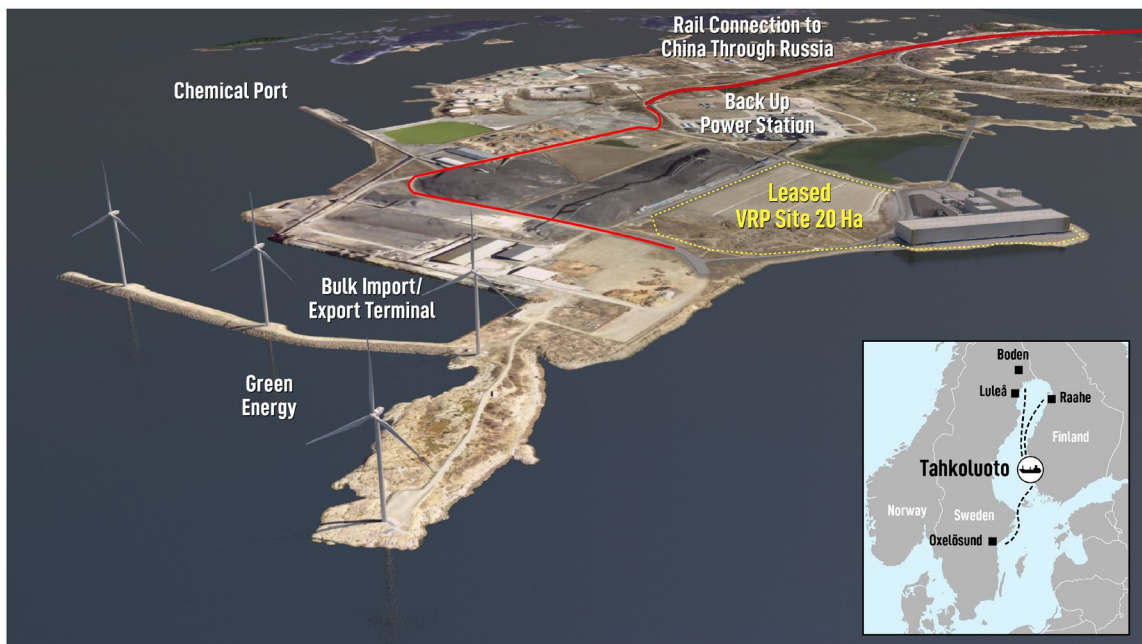
Figure 10 – Aerial schematic showing location for the proposed VRP1 processing plant at Tahkoluoto port, Pori, Finland.
