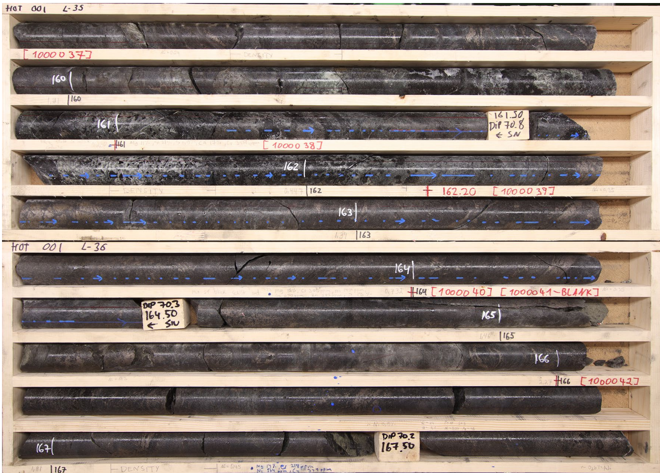
Figure 2. Drillhole HOT001: 159m to 167.9m. Black schist and ultramafic rock with high pyrrhotite content present as blebs, irregular veins and layers.
