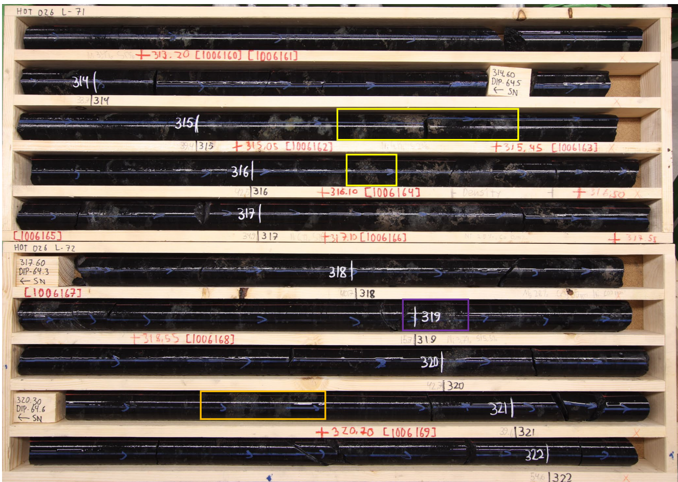
Figure 2. Drillhole HOT026: 312.80m to 322.20m. Serpentinised metaperidotite possessing both intermittent and blebby net-textured and semi-massive sulphide mineralisation (visually, Po > Pn ), intimately associated with metasomatic alteration assemblages with, minor, 1-2% disseminated sulphides throughout.
