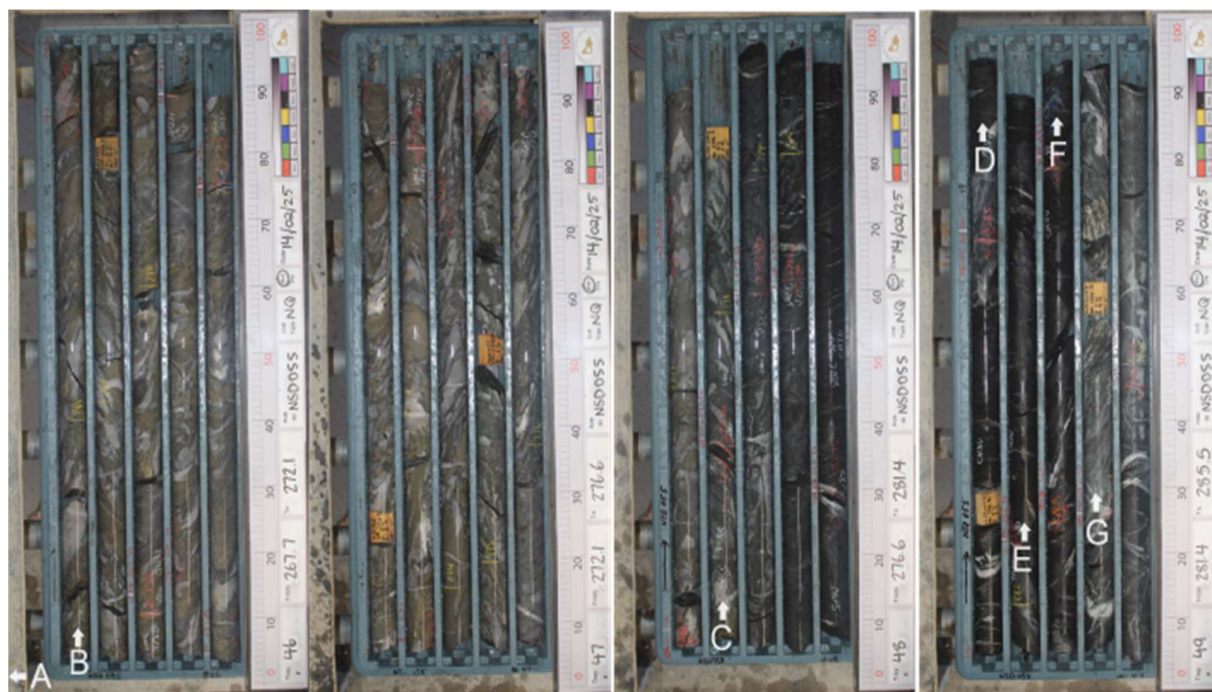
Figure 5 NSD055 276.7 – 285.5m A, Carbonaceous shales (3m up hole). B, weakly sericitised, silica-sulphide altered volcanoclastic. C, Sulphide-silica volcanoclastics. D, Pelite. E, Sulphide-silica volcanoclastics. F, Pelite. G, Basalt. The target horizon is C to end-F. No significant assays. Anomalous mineralisation 280-283.5m.
