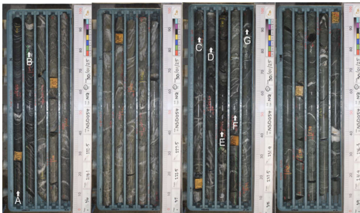
Figure 4 NSD054 218.1 - 236.3m. A, Carbonaceous shales. B, weakly sericitised volcanoclastic. Carbonaceous shales. B, weakly sericitised volcanoclastic. C, Sulphide-silica sediments. D, Volcanoclastic. E, Sulphide-silica sediments. F, Pelite. G, Basalt. The target horizon is C to end-F. No significant assays. Anomalous mineralisation on the contacts above and below the target volcanoclastic sediments.
