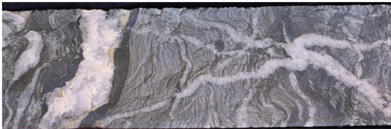
Figure 5 NSD058, mineralised upper contact of interpreted basalt.
