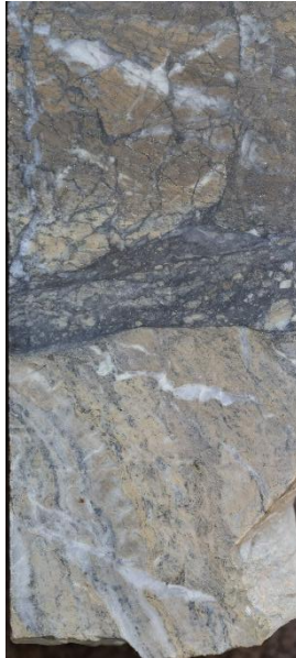
NSD058 – ~283.5m the intercept, although narrow, includes very encouraging geology and structure that indicates the possibility of a Stawell-type gold system.
